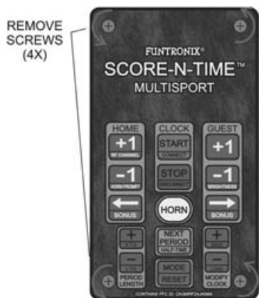
Figure 9.1 Removing the cover screws
