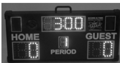
Tournament Mode: Clock, Period, and Score Digits are enabled (no possession arrows)
