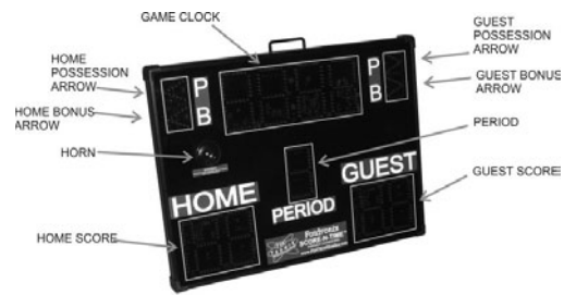
FRONT-PANEL DESCRIPTION OF THE SNT-200M SCOREBOARD
