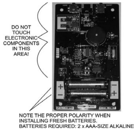
Figure 9b: Removing and installing new batteries
